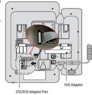
Connect one of the data cables supplied with the EHS Adaptor between the EHS Adaptor and the EHS Base Set.
